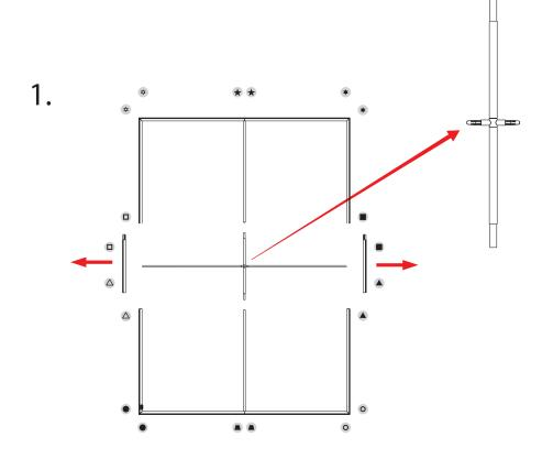
Remove Center Extrusion and Cross Bar Connector
